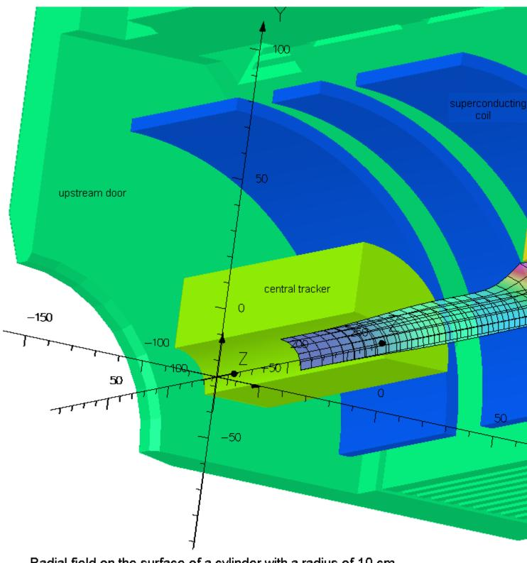
Radial field on the surface of a cylinder with a radius of 10 cm. Maximum field towards the top edge of the aperture of the downstream door (red/pir
