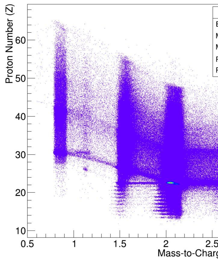
FRS PID - <sup>46</sup>Ti Setting (After Scintillator
