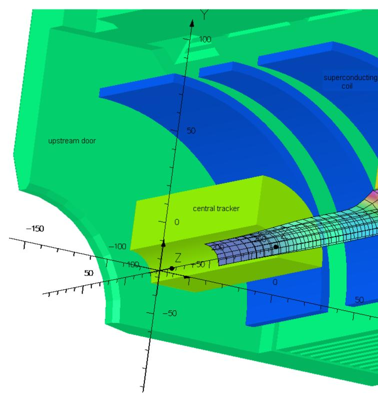
Radial field on the surface of a cylinder with a radius of 10 cm.
