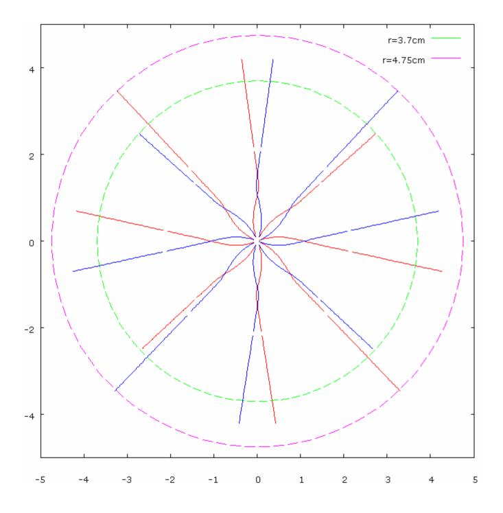
Protons and antiprotons (red/blue, momentum 1.5 GeV/c) emitted under 5 mrad from the IP.
